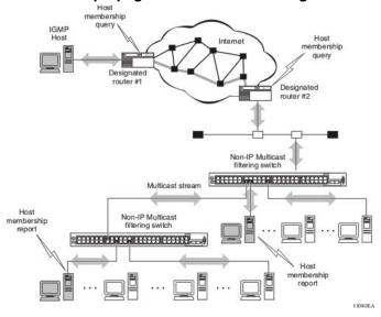
The Nortel Ethernet Routing Switch 5500 Series can automatically set up IP Multicast filters so the IP Multicast traffic is only directed to the participating end nodes (see ).
